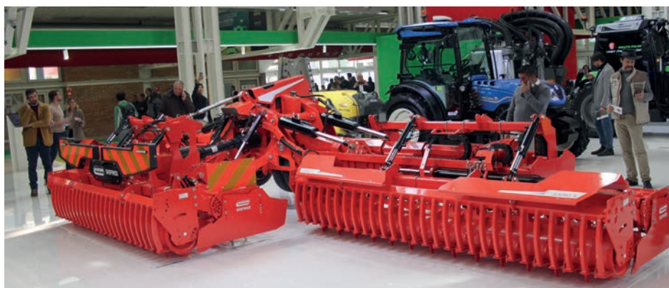
Maschio Gaspardo's Jumbo X design takes power harrows into 10m working width territory for the first time.
