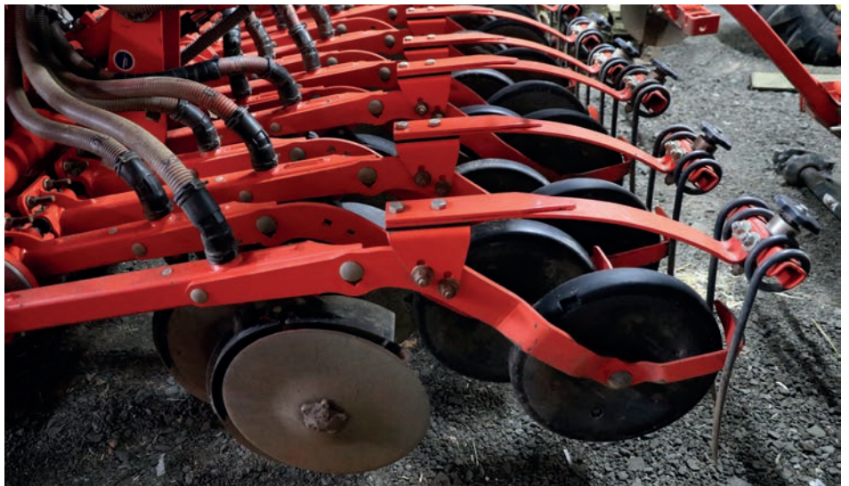
The Espro's row of press wheels are in front of the coulters rather than behind, as is the case on some other models.
