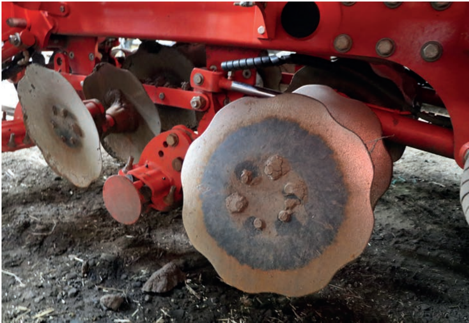
The Espro's coulters design has two angled discs which are slightly offset to allow soil to flow easily through and limit disturbance.
