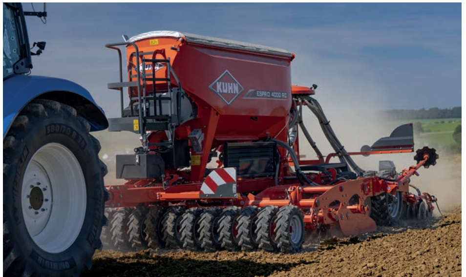
The Kuhn Espro is a universal seed drill which is designed for use after ploughing, minimum tillage or directly into crop residues.
