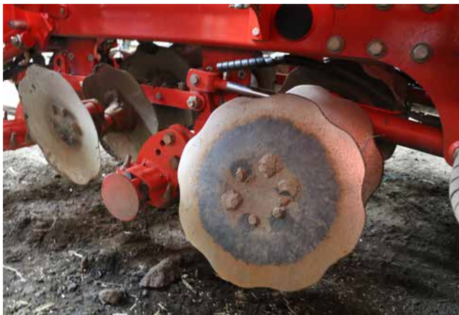
The Espro's coulters design has two angled discs which are slightly offset to allow soil to flow easily through and limit disturbance.
