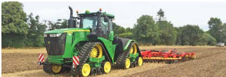
One of the key differences when FW Rowe and Sons switched to tracks was how the tractors were suddenly more capable of pulling everything while causing less compaction.
