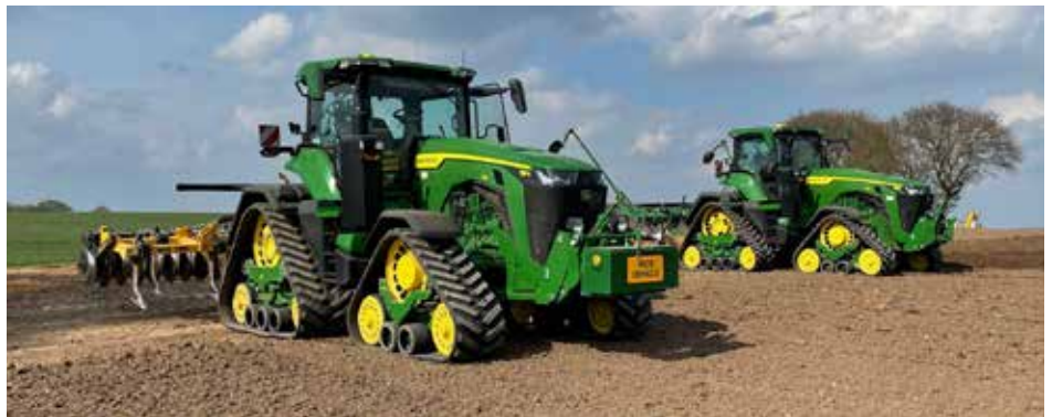
Tracks have negated the necessity to add, remove or change ballast weights every time a different piece of equipment is used at FW Rowe and Sons.
