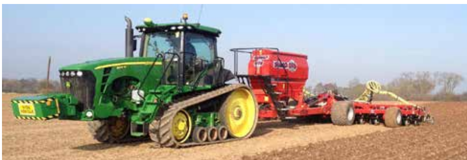
Care is taken at FW Rowe and Sons to ensure the tracked machines are kept on top of firm land and not run in furrows which they’re not best suited to.
