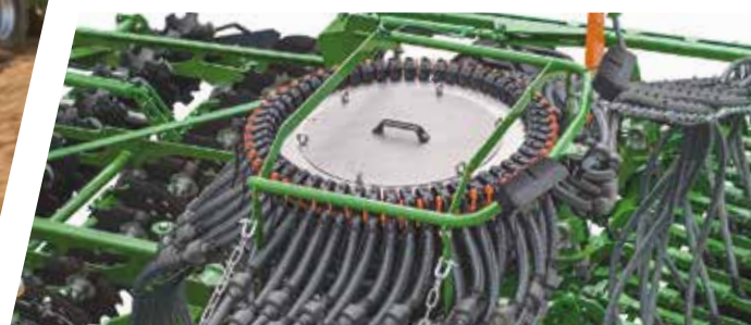
The individual row shut-off distributor head can also easily work with any symmetrical or asymmetrical tramline systems.
