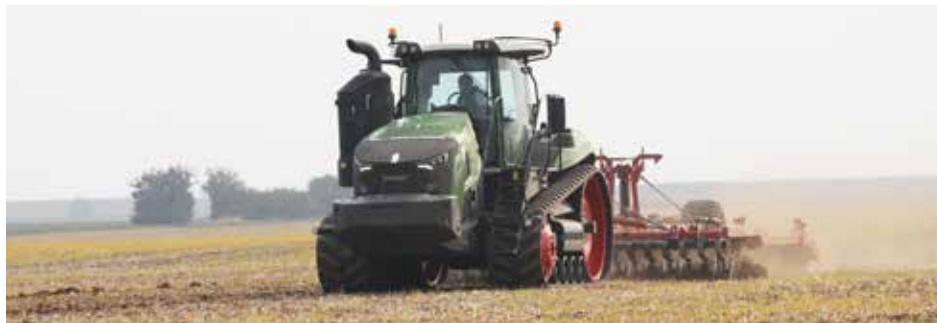
The Fendt 1162 MT covers 600 hours per year with one of its main jobs pulling a 5m Keeble Progressive cultivator at J D Mee and Son.
