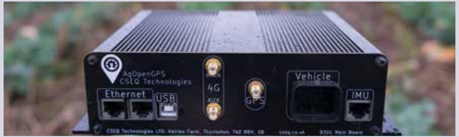
‘Box 3’ – marketed by Charles’ business, CSEQ Technologies – is a streamline system comprising the control box, hydraulic valves, antenna and a Windows tablet which comes pre-loaded with the software.
