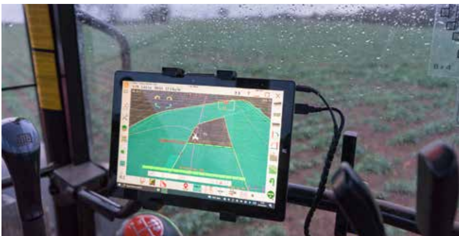
The software that powers the kit is AgOpenGPS – a global network of GPS guidance software built by farmers.
