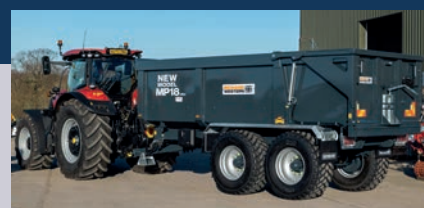
The MP18 body is constructed from Hardox steel to reduce weight and increase strength, while enhancing wear resistance above the high-grade steel used in the Richard Western's other trailers.
