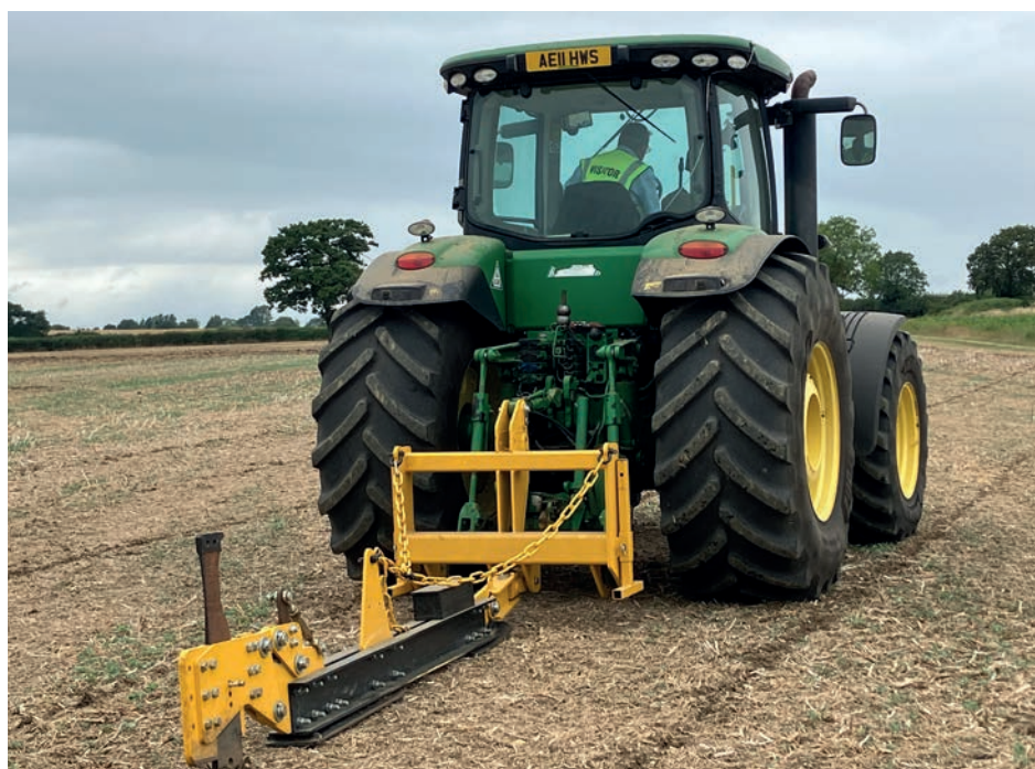
Mounted on the tractor’s rear three-point linkage, the Claydon Mole Drainer features an oscillating headstock.
