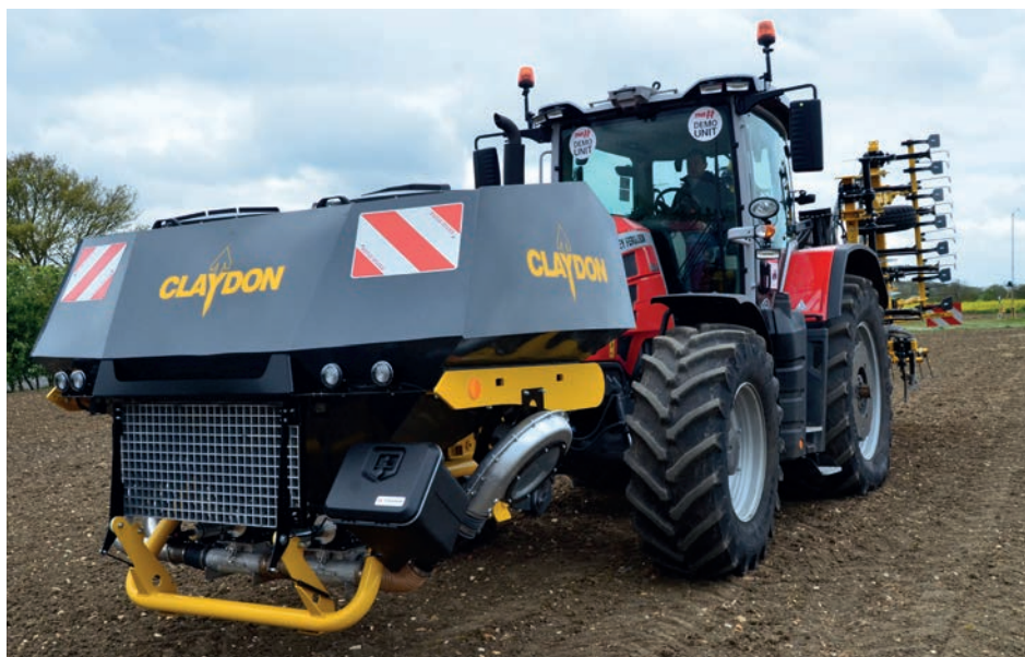
Claydon’s most recent product development is this front tank/rear 3-6m toolbar version of the Evolution mounted drill.
