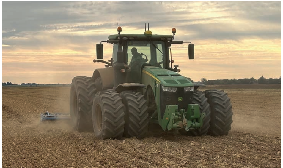
A John Deere 8R tractor was fitted with wider BKT 900mm rear wheels with BKT 710mm front wheels to support the heavy front axle, thereby decreasing compaction and increasing traction.
