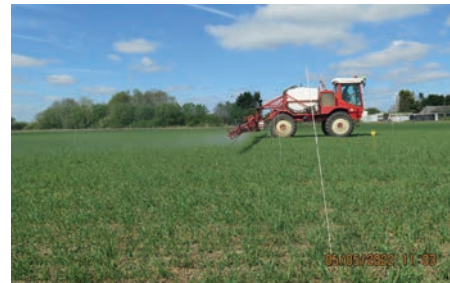
Independent trials carried out in 2022 have looked at the impact of four different nozzle types – Lechler ID3, Hypro Guardian Air, Hypro 3D and a 110 Fan Jet – on glyphosate application and performance.
