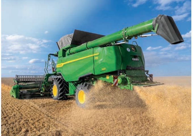
John Deere's T5 and T6 combines have new grain tank options including a 13,500-litre tank option on the T6 and an 11,500-litre tank on the T5.
