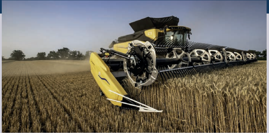
The New Holland CR11 runs a 16-litre FPT Cursor engine capable of generating 775hp and has a 20,000-litre grain tank.
