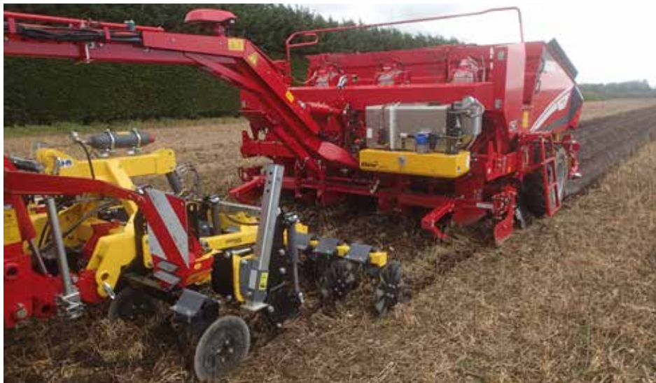
The aim of the Grange toolbar is to zone cultivate where required with a leg in line with where the potatoes are being planted.
