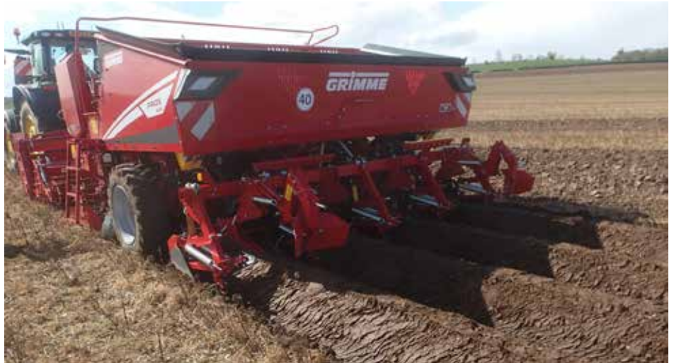
Grimme has provided the project with a new Prios planter for less passive sliding and more rotating disc type action which moves the soil during ridge formation.
