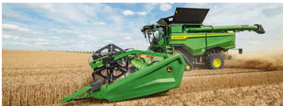
Residue management on the S7 combine has been updated in line with the X9 concept so it's mechanically driven.
