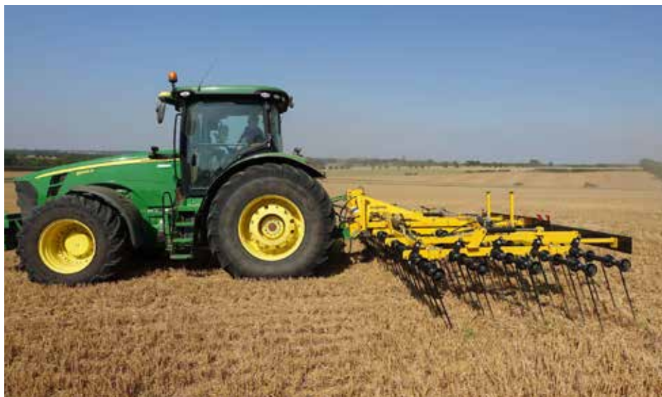
Jeff Claydon quickly became convinced of straw harrowing’s ability to incorporate material into the surface, helping worms to harvest it, while also destroying slug eggs and weed seedlings.
