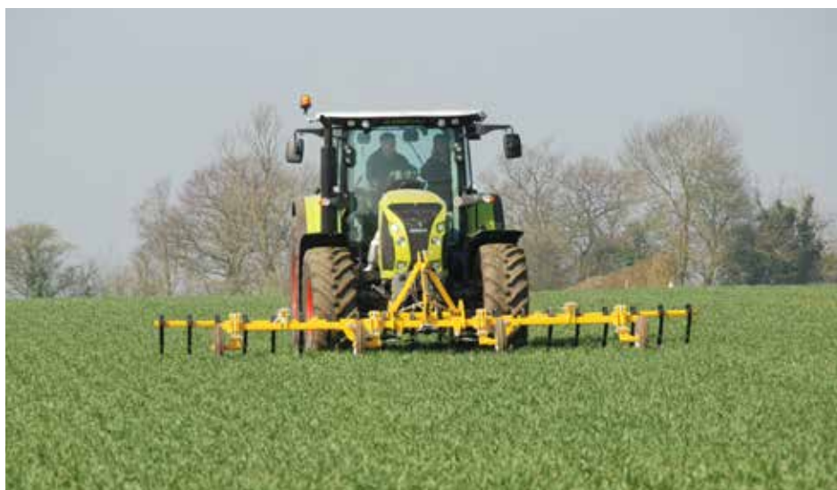
With the Claydon system’s ability to sow in bands, in 2015 the firm launched the Terrablade as a simple tool for mechanical weeding between rows.
