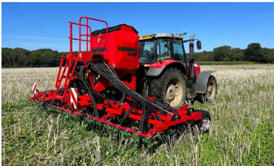
Dale Drills' Mounted Tine Drill (MTD) now offers a split tank feature enabling simultaneous sowing of two different seeds or products.
