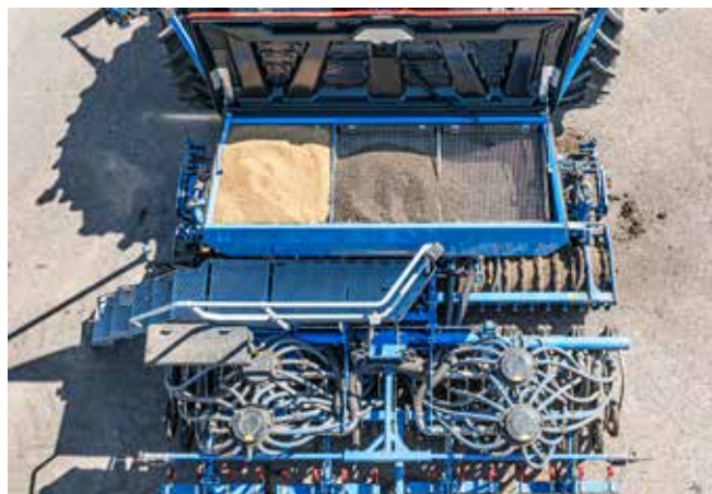
The Lemken MR series features a 1500-litre tank which is suitable for fertiliser even in its basic configuration.
