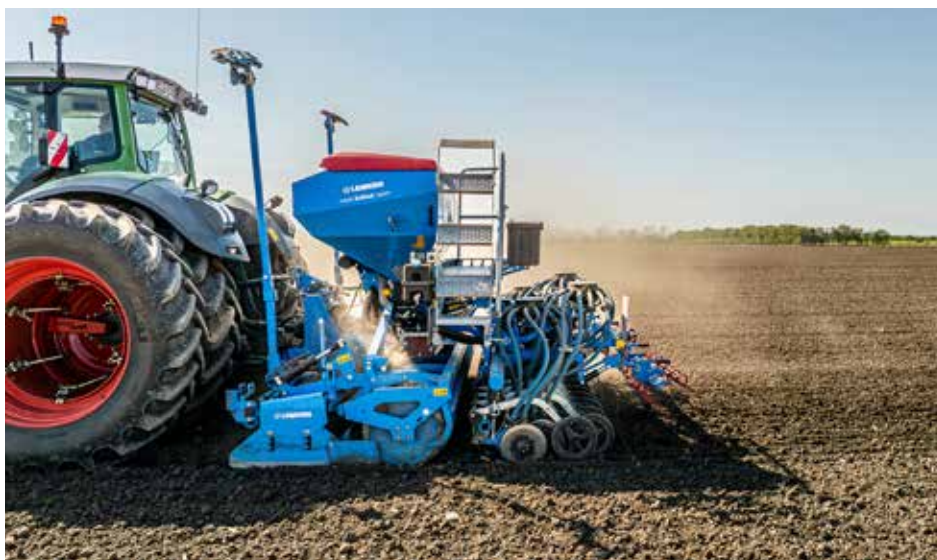
The new mounted Lemken Solitair with a working width of 3m and 4m is equipped for both conventional and conservation tillage.
