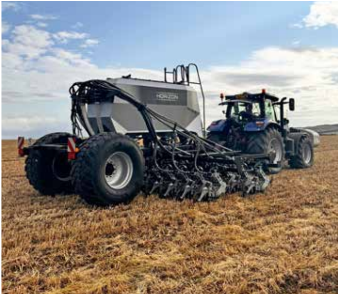
The parallelogram on the front of the Horzion DSX mounts onto the frame, has 32cm of individual travel per row unit and hydraulic downforce of up to 300kg if required.
