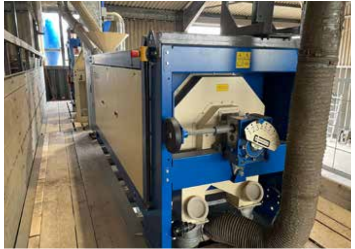
The Intercropper is paired with a JK Machinery Indented Cylinder which conducts a second finer separation of the smaller crop based on shape.
