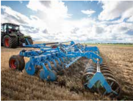
Lemken has introduced the 10m wide Rubin 10 to round off the top end of its range of the Rubin compact disc harrows with a large disc diameter of 645mm.
