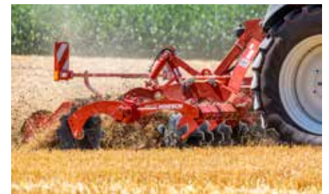
Horsch's new Joker RT has been designed for stubble cultivation, mixing of harvest residues and efficient seedbed preparation.
