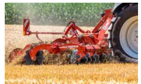
Horsch's new Joker RT has been designed for stubble cultivation, mixing of harvest residues and efficient seedbed preparation.
