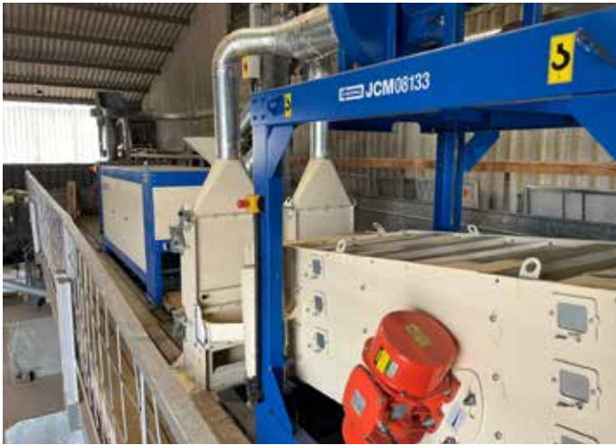
The machine has both pre- and post-aspiration to remove light admixture and dust, but the real separation happens on the three sieve decks.
