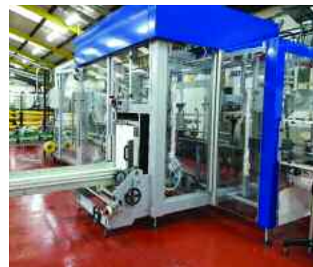
Recent additions to FMC Pentre include a semi-automated filling machine to help reduce manual handling.
