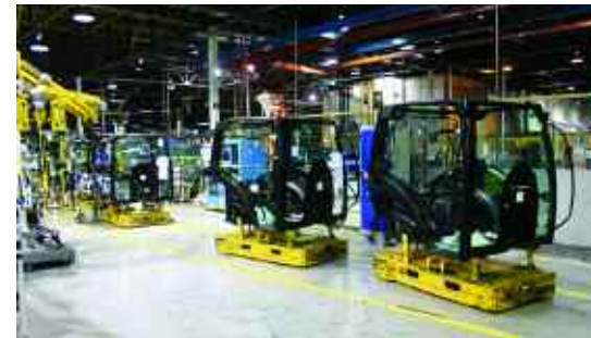
Cabs frames from the Croix plant in France are trimmed and finished at Basildon as part of tractor assembly.
