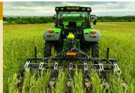
Andy Cato's interrow mower design has been replicated for others in the Wildfarmed community, who are using it to manage different kinds of relay-cropping systems. Photo: Andy Cato, Wildfarmed.
