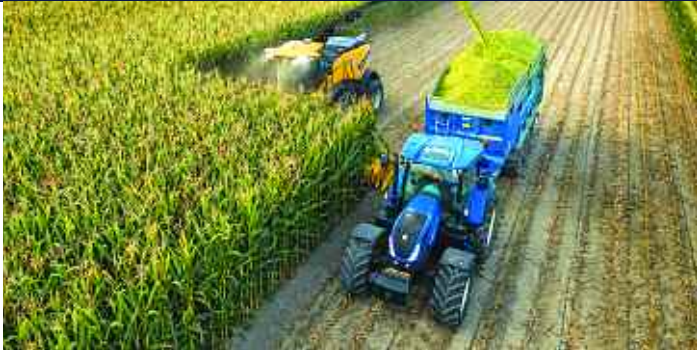
Attractions of the larger FR920 included more heavily-built components and the use of Hardox steel all the way through the key wearing parts, including the drum, blower, chute and spout.
