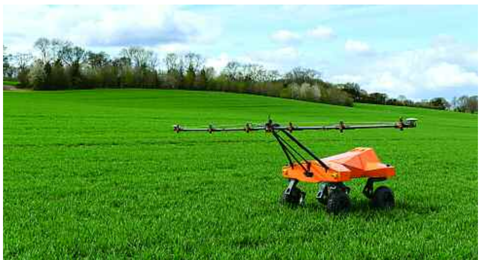
The 'Tom' scouting robot uses imagery and AI to geolocate and analyse plants at millimetre accuracy.
