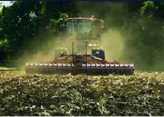
The Väderstad TopDown for shallow working or the Sumo Quatro for deeper loosening are both followed by a 10.5m Väderstad Rexius Twin press where necessary.
