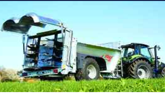
Fliegl's ADS push-off manure spreader combines its push-off technology with powerful spreader mechanisms for solid manure application.
