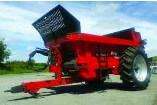
Agri-Spread's VB Pro range is offered in six capacities/models from 6-12t single axle models.
