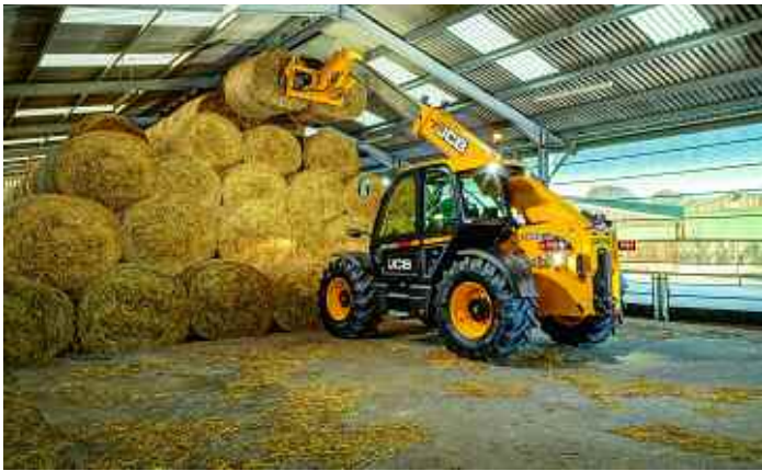
The JCB Agri Pro has a 4.8-litre JCB DieselMax engine in the Pro also delivers 690Nm of torque at 1500rpm.
