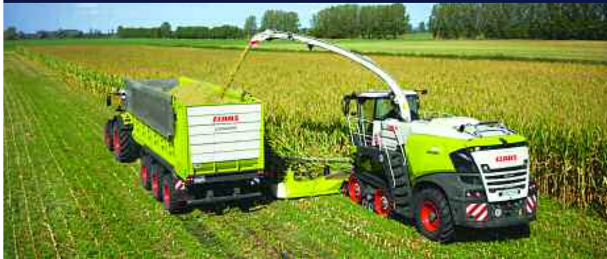
Claas' Jaguar Terra Trac is the first self-propelled forage harvester available with a factory-integrated crawler track system with hydraulic suspension.
