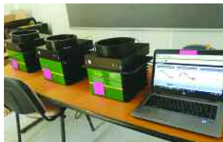
The John Deere HarvestLab 3000 NIR sensor can be removed from the forager chute and used for stationary analysis.
