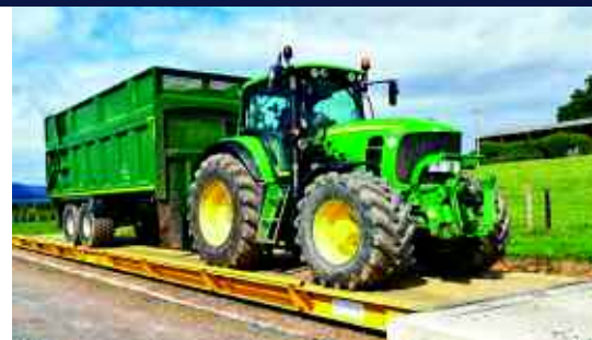
Counting and weighing silage trailers on a weighbridge was one of the five testing methods used in the ADAS Grass YEN field trials.
