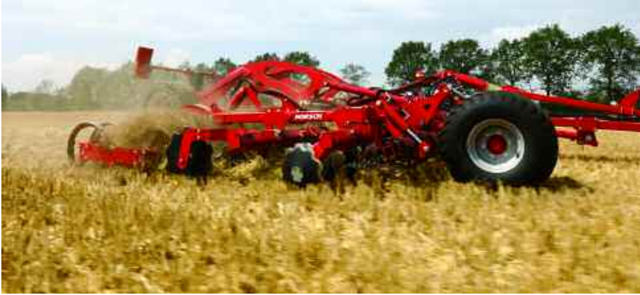
New from Horsch is the Joker CT and RT disc harrows, designed for stubble cultivation and seedbed preparation.
