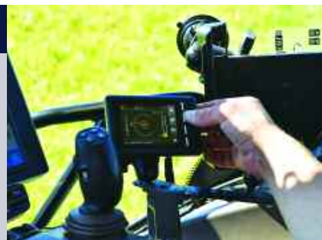
Quicke's new Q Companion uses sensors mounted on the loader to accurately weigh the contents lifted by an implement.
