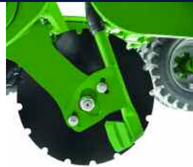
The FerTeC coulters apply the fertiliser in front of and slightly below the seed coulters.
