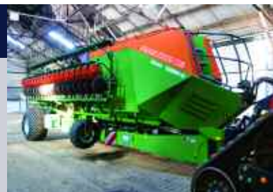
The Citan drill with RoTeC coulters ensures minimum disturbance in the CTF system.
