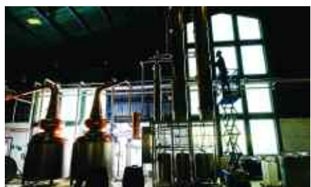
The two tall copper columns distil the pure spirit, while it's the shape of the still, along with choice of raw materials and distiller's art that defines the taste.
