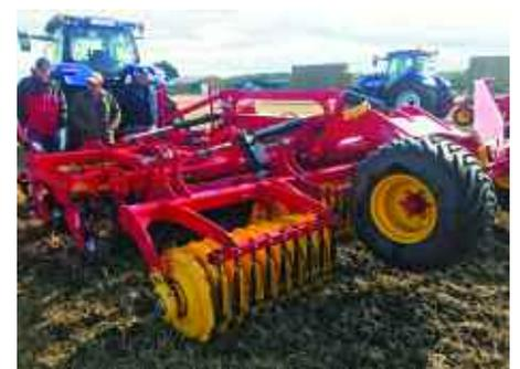
Operating at ultra-shallow working depths of between 2-3cm, the CrossCutter disc is claimed to move substantially less soil than a conventional disc.
