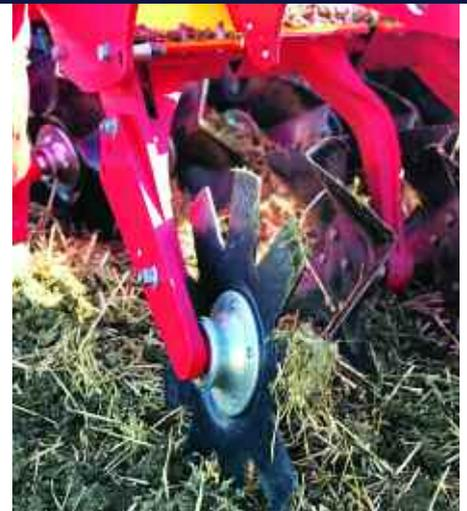
The CrossCutter disc is fitted to the Väderstad Carrier disc cultivator and is individually mounted to its own rubber suspended disc arm.
