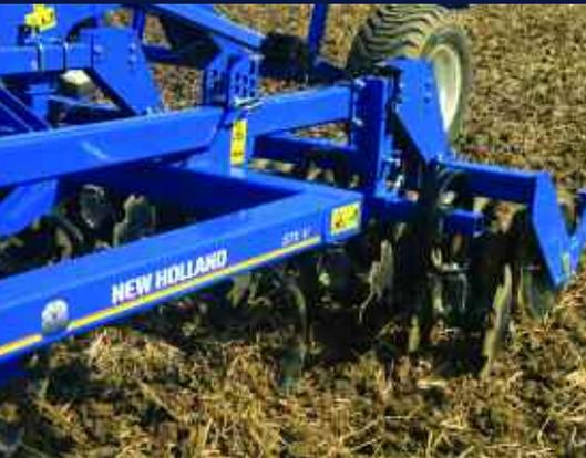
According to New Holland the STX V is an 'all-rounder' which is suitable for conventional stubble operations as well as those looking for mulch tilling.
