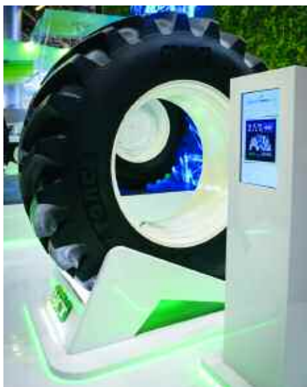
The casing structure of the Agrimax Froce is designed to provide maximum sidewall flexibility.
