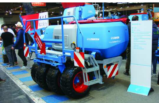
Lemken's Solitair 23 front tank holds 1900 litres of seed which can be fed to a rear-mounted coulters bar or precision seeder.
