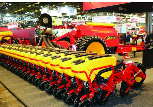
Väderstad now has a new eight-row model at the base of its Tempo L range, offering 700-800mm row spacing, although it can also be configured as a 12-row machine.
