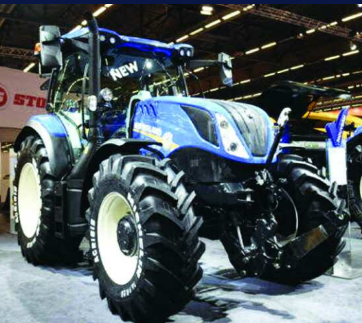
New Holland's new 135hp (rated)/165hp (max) T6.160 is an alternative to the four-pot T6.165, which has the same power figures.
