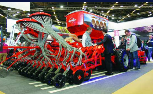
Kuhn's Aurock drill is available with a split hopper and dual metering, enabling establishment of two different crop types at different sowing depths.
