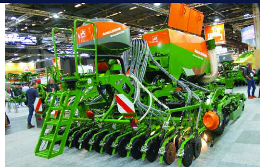
The latest addition to Amazone's Cirrus cultivator drill range is the 4/6m CC variant, which has a 4000-litre 60/40 split hopper.
