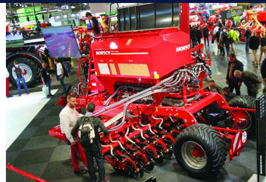
The Horsch Avatar SD single-disc direct drill range can now be equipped with a three-way split tank and place three different products concurrently.
