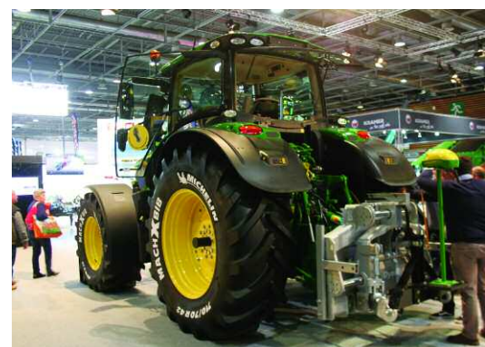
Displayed on the John Deere stand was hitch specialist Laforge's Dynatrac universal guidance interface, which keeps implements on track.
