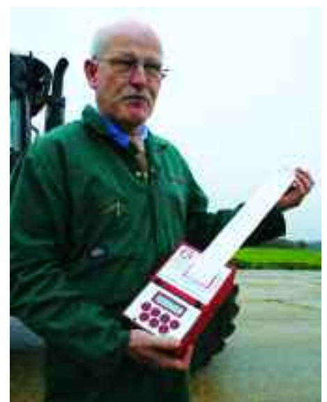
Agricultural engineering consultant Andy Scarlett with the BrakeSafe device that machinery dealers use to test tractor and trailer braking performance.
