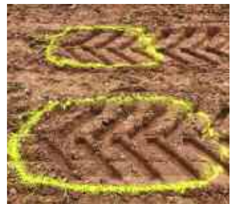
The difference in footprint size can be considerable when you compare incorrect (top) and correct (bottom) pressures on the same vehicle, same tyre and with the same load.
