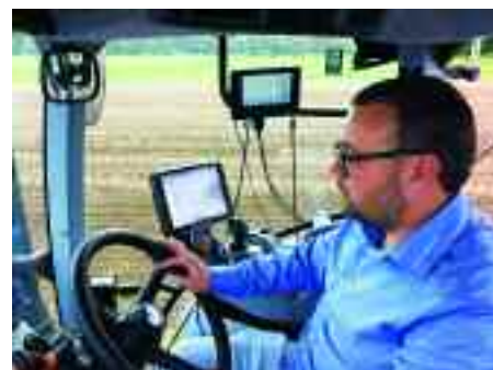
In the cab, the only noticeable difference is the tablet showing the tractor’s course and the points at which readings are taken.
