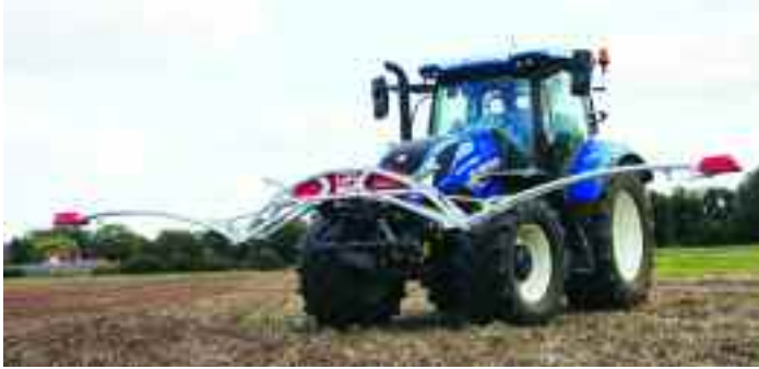
Other precision tools from CNHi include the Crop Sensor boom, which uses optical sensors to measure crop nitrogen need and alter application rate of a rear-mounted fertiliser spreader.
