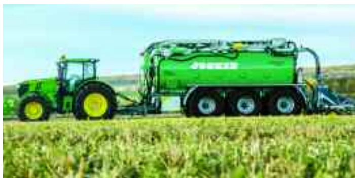
Fit John Deere's HarvestLab NIRS analyser (yellow box) on a Joskin slurry tanker together with some other hardware and software and application rate in terms of kgN/ha can be regulated automatically.
