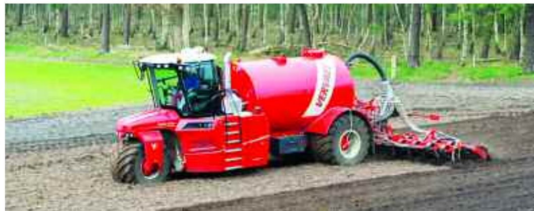
The Vervaet Hydro Trike self-propelled tanker can also operate with the John Deere HarvestLab unit to provide automatic pump output control.
