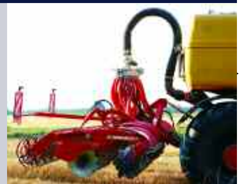
Vogelsang SynCult conversion kit is available for a number of short disc harrows, including the Horsch Joker short disc cultivator.
