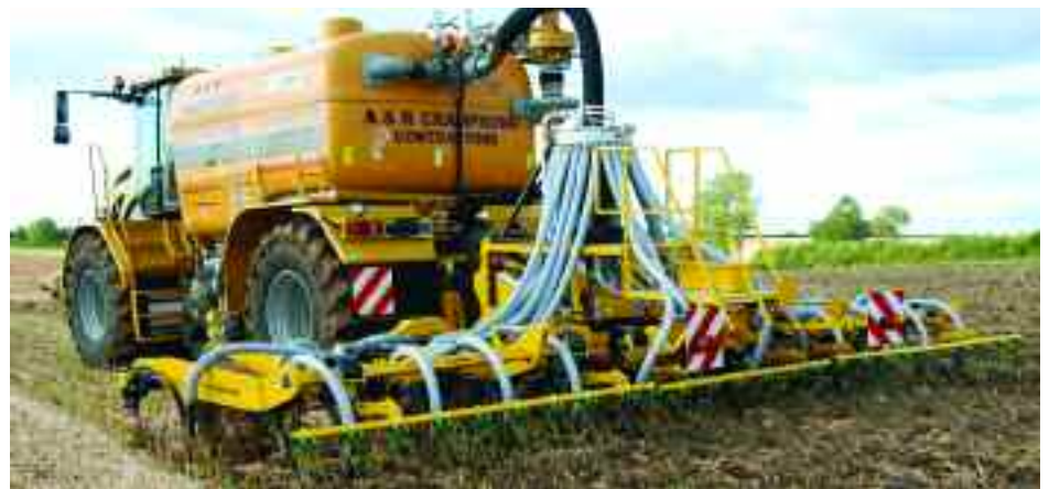
The Claydon Injector uses the familiar two-tine arrangement from the company's drills at 30cm or 60cm spacing.
