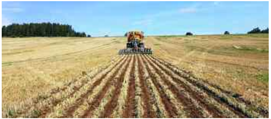
The XTill provides strip cultivation and slurry or digestate injection prior to precision sowing maize – a one-pass oilseed rape seeding system is also available.
