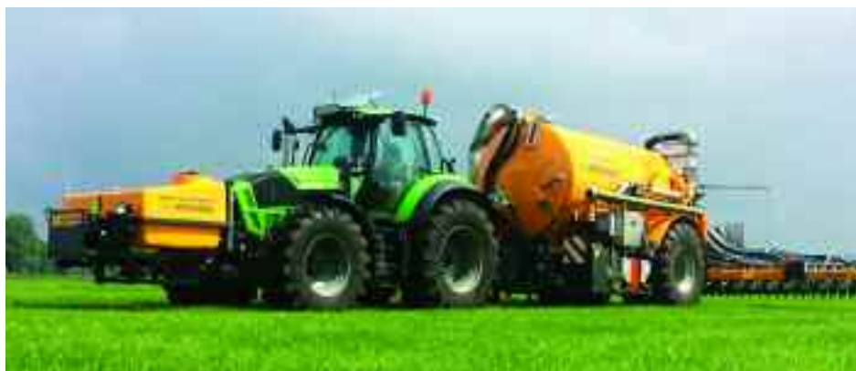
The Veenhuis Nutri-Flow system analyses nutrient levels in each batch of slurry or digestate as the tanker is filled, with a supplementary shot of liquid fertiliser supplied from a front-mounted tank.
