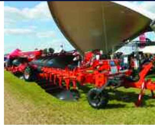
Kuhn's Smart Ploughing package is a section-control system that uses GPS guidance signals to progressively lower and lift individual plough bodies automatically.
