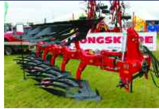
Kongskilde’s XSD slatted body is based on the profile of the established XLD conventional type, designed for use up to 710mm tyres.
