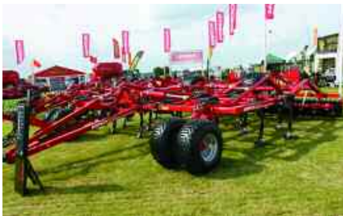
Depending on configuration, Horsch sees its Terrano GX as suiting jobs ranging from loosening compaction to intensive mixing of trash and soil.
