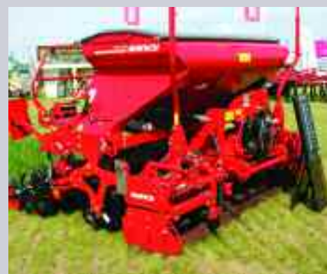
Horsch's Express KR is claimed to be the first singulation drill on the market suited to establishment of wheat, barley, OSR and peas.
