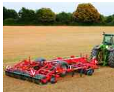
The Performer 5000 is the mid-range model in Kuhn's non-powered, deep working disc and tine cultivators, with a working width of 5m.
