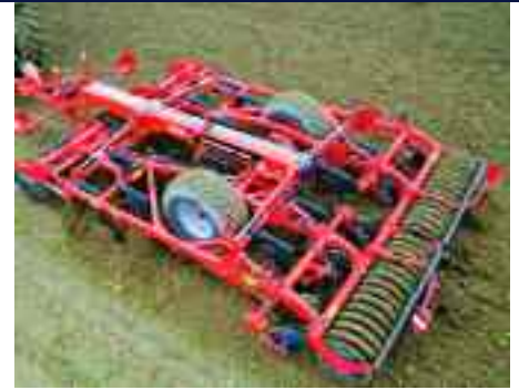
The machine is fitted with 38 discs and 18 tines, designed to work to a depth of 10cm (discs) and 35cm (tines).
