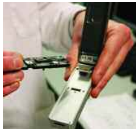
Real-time sequencing can be done in the field with the Nanopore MinION – the kit with disposable flow cells is available to buy on the internet for $1000.
