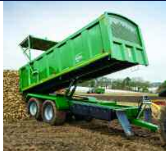
Long reach cylinders achieve 60 degrees of tip on Bailey new Beeteaper model.
