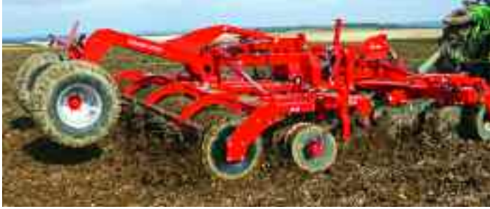
The 5.5m Combi Disc can subsoil, surface cultivate and consolidate in a single pass.
