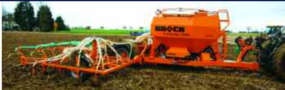
The Brock Campaign 900S has a working width of 13.4m.
