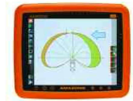
With WindControl the entire spread fan is constantly monitored on both sides by 14 radar sensors.
