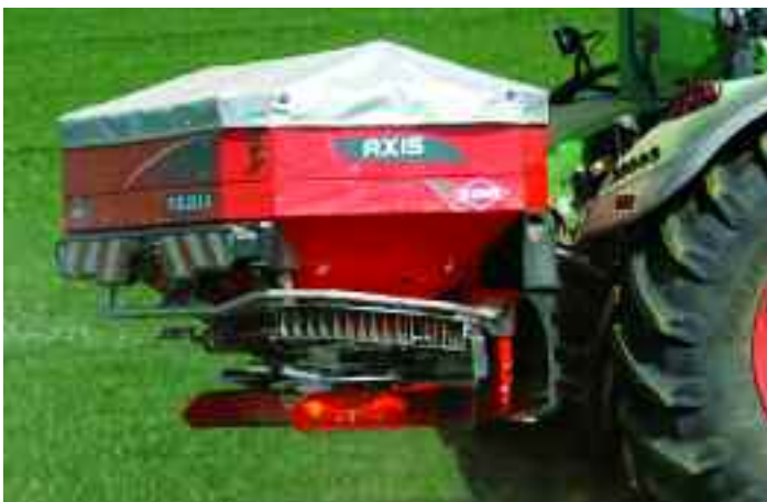
SpeedServo introduces a rotational action to accelerate the metering and drop-point adjustment process by 2.5 times.
