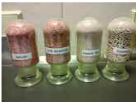
The various forms of kieserite, from the crude rock salt (left) to the granular form (right) that's well matched with ammonium nitrate or NPK blends.
