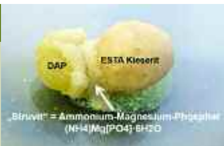
If DAP and Esta Kieserit are placed next to each other, struvite can be naturally formed.
