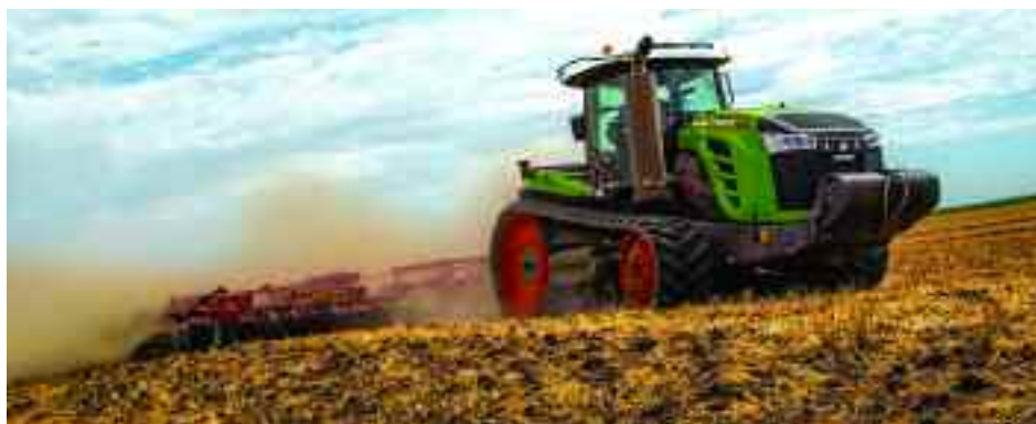
Fendt 900 Series tracked machines are the first to have a fully suspended cab.
