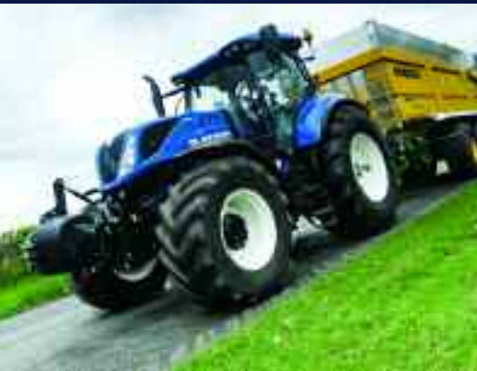
Tractors in the T7 180-240hp class have a new front axle and steering control for precise operation at speed.
