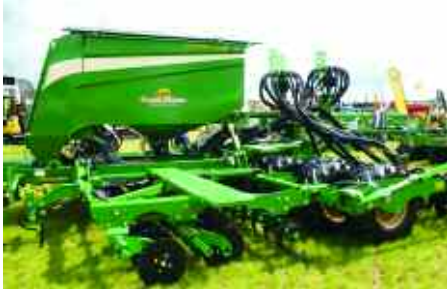
Great Plains has added a new 6m wide grain only version of its Saxon drill, while 3m and 4m versions have grain and fertiliser options.
