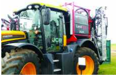
Landquip's demount unit for the new JCB Fastrac 4000 has a new 30m boom, which folds vertically behind the machine.
