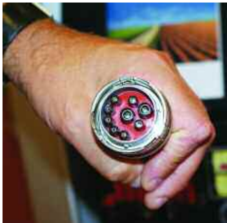
Plug an implement into the ISO 11783 socket and the iMonitor recognises it, populating the screen with essential operating information.
