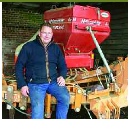
Dan Kiddy has modified a Simba Flatliner five-leg subsoiler with a seeder unit and low-disturbance points and double rolls to lock in moisture.
